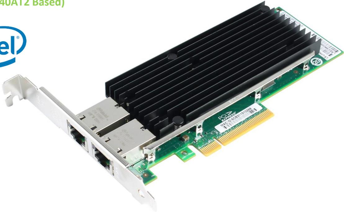
**10GBASE-T converged network adapter simplifies migration to 10 GbE, provides iSCSI, FCoE, Virtualization, and Flexible Port Partitioning.**
